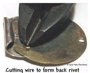
12. Cut the wire, close but not flush to the metal. You need only a small portion sticking up.
