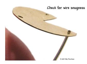
6. Once your holes are all drilled, place your wire through the holes to make sure you have a snug and tight fit. You may have to twist the wire to get it in or if that doesn't work, use a round tapered jewelers file to file the hole a little until the wire fits.
