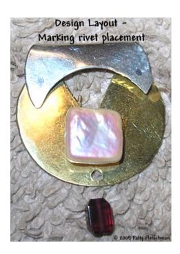
2. Then mark the top piece with a pencil or marker, where you want to drill the holes to place the rivets. (Sometimes with the right design you can tape the two pieces together because it is easier to drill both pieces at the same time, so you are, spot on, with your holes.)
