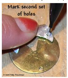
3. Place your first piece on a wooden block. Take a steel punch and place it on the marks you made and tap it with your hammer to make an indention. This is done so that when you place the drill bit on the metal and begin to
