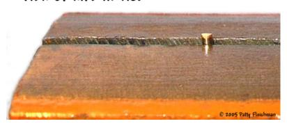
8. Take the ball end of your hammer and gently tap the edges of the end of the wire in a circle. You keep doing this until you see a head develop on the end of the wire. If you hit the wire too hard it will bend it and you don't
